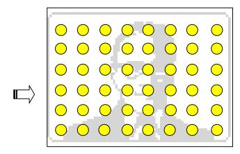
The user needs to see the situation in each channel in order to set a detection zone within the 8W ×6H (48) area. The effective points are marked " " $\bigcirc$ " (yellow).
